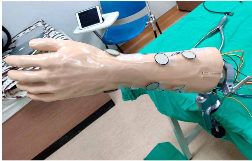
Figure 4. The simulated arm was fixed to a clamp which was mounted to a bench top.
