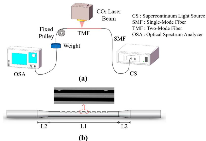
**Figure 4.** (a) Schematic diagram of the BLPPFG preparation. (b) Schematic diagram of the BLPPFG and photomicrograph of one period in the taper waist.
