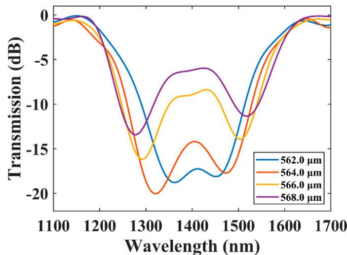
Figure 5. The transmission spectra of BLPFGs. The cladding diameter is 121  $\mu\text{m}$ , and the periods are 568.0  $\mu\text{m}$ , 566.0  $\mu\text{m}$ , 564.0  $\mu\text{m}$ , and 562.0  $\mu\text{m}$ .
