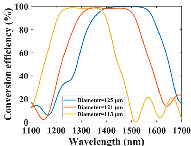
Figure 6. The conversion efficiency of three BLPFGs with a diameter of 113  $\mu\text{m}$ , 121  $\mu\text{m}$ , and 125  $\mu\text{m}$ , respectively.
