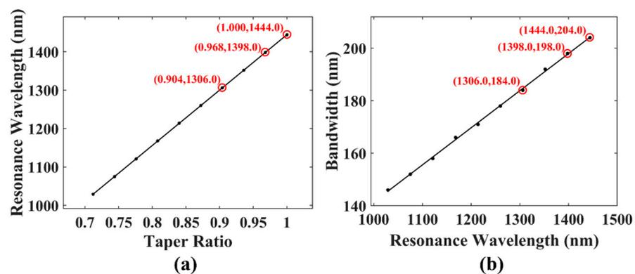
**Figure 3.** (a) The change in the dispersion turning point with the taper ratio. (b) The change in the 15 dB bandwidth with the dispersion turning point.
