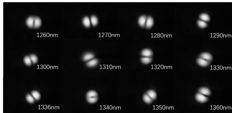
**Figure 7.** The output modes of the BLPFG in its working window.
