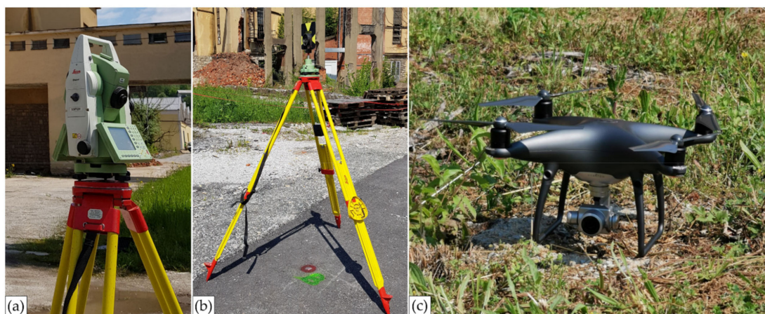
Figure 4. Geodetic sensors and accessories used in this research; (a) total station (TS) Leica Geosystems TCRP1201+ R400; (b) survey accessories: tripod (Leica Geosystems GST20); tribrach (Leica Geosystems GDF322); reflector carrier (Leica Geosystems GRT144); reflector (Leica Geosystems GPR121); (c) unmanned aerial vehicle (UAV) DJI Phantom 4 Pro.
