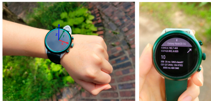
Figure 2. Smartwatch system with its axes displayed (left), and a screen from the running application created to capture dynamic hand motion (right).
