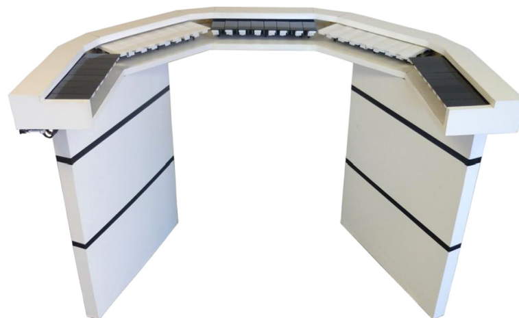
Figure 8. The Vibrochord, a vibrotactile musical input device VMID, retrieved from [66].
