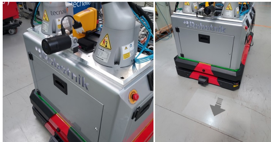
Figure 5. Projector installed on robotic platform to display the direction to the next path pose.
