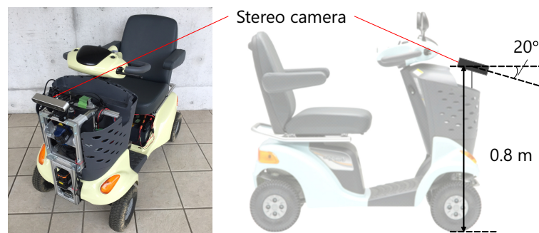
Figure 6. Experimental vehicle and sensor mounting position.
