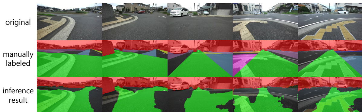
Figure 19. Inference results of trained model after loss weight adjustment with 50 \times 225 + 400 \times 50 cropping.
