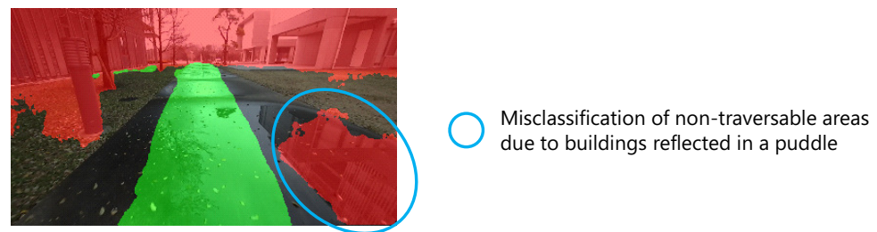
Figure 20. Example of misclassification of non-traversable areas due to non-traversable objects reflected in a puddle.
