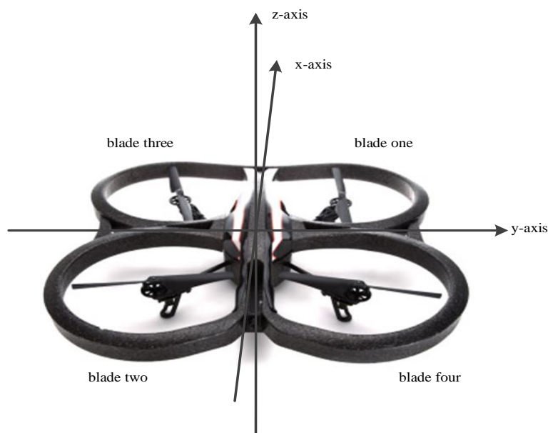
Figure 6. The structure diagram of the quadcopter and the x, y, and z-axis regulations.
