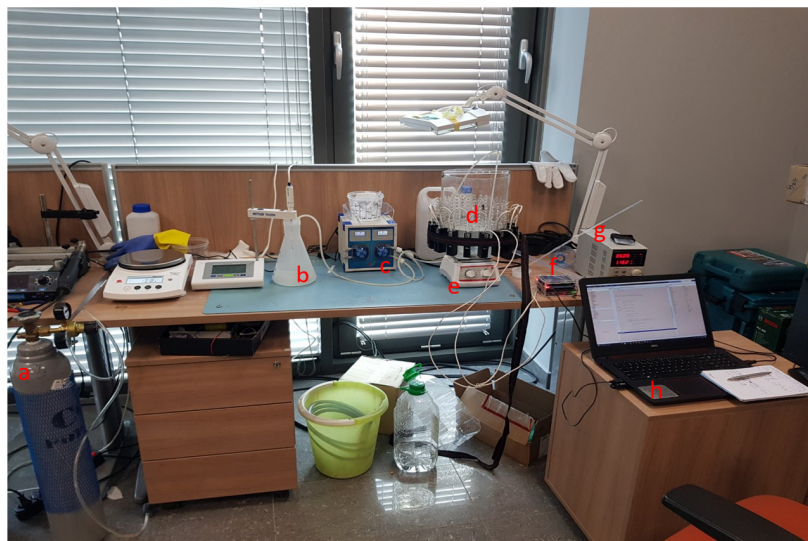
Figure 8. Photo of the batch crystallisation experimental apparatus. (a) Carbon dioxide tube for gas injection; (b) reagent vessel filled with sodium carbonate solution (reagent); (c) electronic peristaltic pump; (d) receiving tank filled with calcium chloride solution; (e) IKA Midi 1 digital magnetic stirrer; (f) tomographic device developed by NETRIX company; (g) power supply; (h) computer unit used for running MATLAB code and providing tomographic results.
