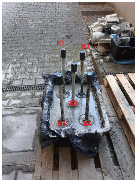
**Figure 14.** Laboratory model of bolted roof.
