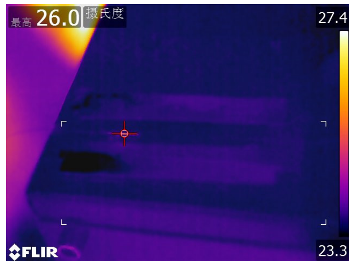
Figure S5. Infrared photograph of MNF deposited on tin oxide film, the red cross is the highest temperature area within MNF and the guided light direction is from left to right.
