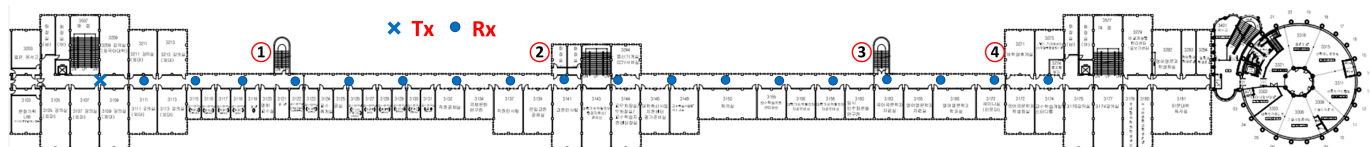
Figure 3. The experimental outlet is on the 3rd floor of the main building corridor. Structures that create irregularities in the corridor are marked with circled numbers: ①; ②; ③; and ④.
