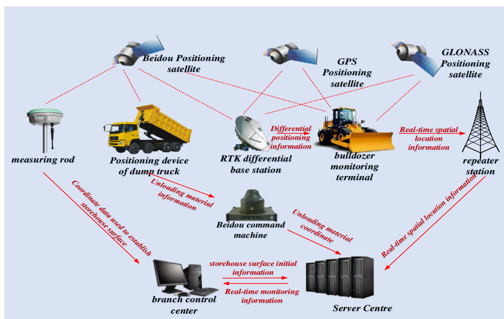
Figure 8. Real-time acquisition process of paving operation parameters.
