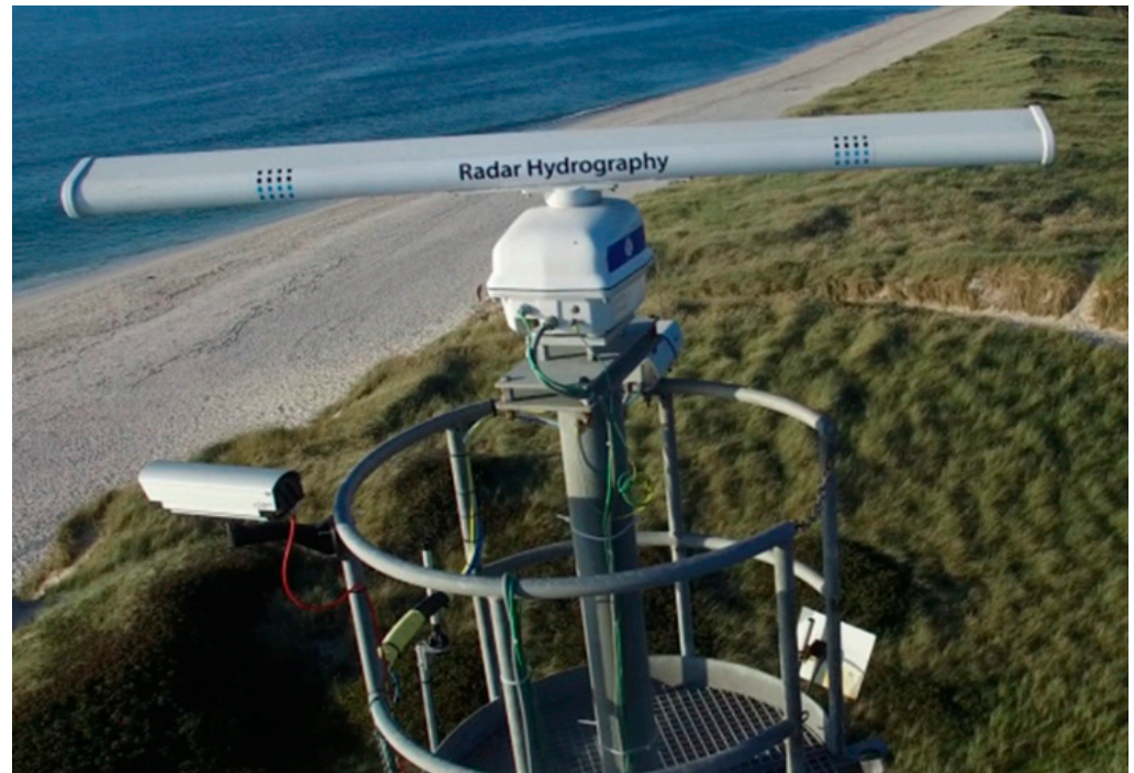
Figure 1. Coastal setup of the coherent on receive marine radar (MR) system on the Island of Sylt in the German Bight of the southern North Sea.
