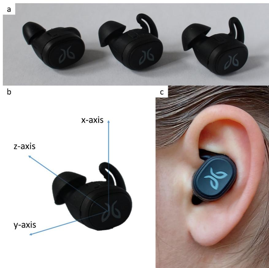
**Figure 2.** Instrumented wireless earbud. (a) Three earbuds with differently sized attachments. (b) The coordinate system of the accelerometer in the earbud. (c) The snugly fit earbud in the ear.
