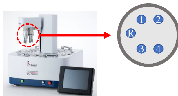
Figure 3. Taste sensor system TS-5000Z. One measurement cell could contain at most 4 sensor electrodes and 1 reference electrode. The 4 sensor electrodes do not need to use exactly the same membrane. In this study, the membranes used in the 4 sensor electrodes of one measurement cell were the same in measuring the samples and calculating the standard deviations.
