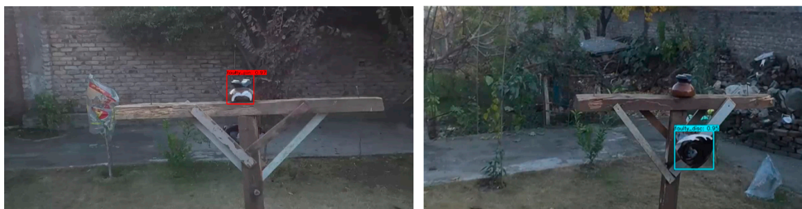
Figure A5. Test results of the proposed YoloV4-based faulty insulator detection model with flight path patterns.
