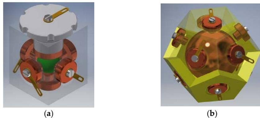
**Figure 12.** Tilt sensors based on the Platonic solids: (a) cuboidal sensor; (b) dodecahedral sensor.
