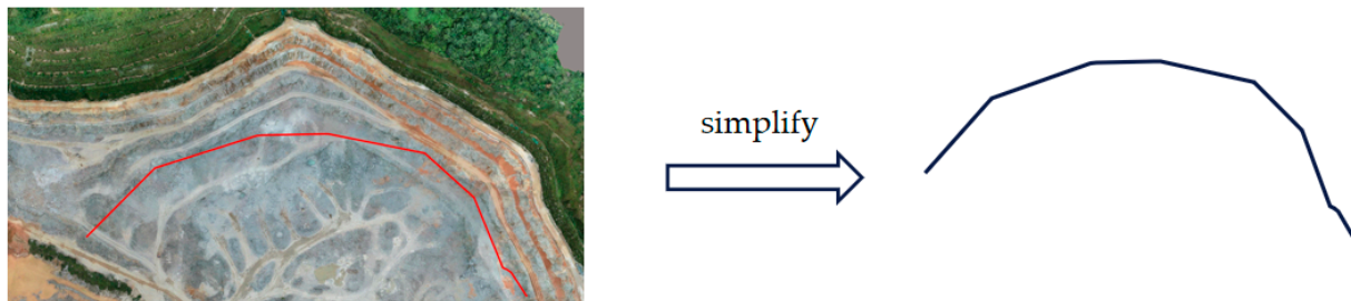
Figure 6. Mine surface simplification: in the XY flat, closest to the camera is the slope line where the red curve in the diagram is located. The closer the distance, the smaller the camera's sensing range. If this line can be fully covered, other heights of the slope must be covered, so we have chosen this line to represent the situation of the mine surface in the XY plane.
