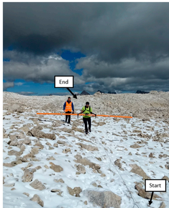
Figure 4. Picture taken during the FDEM measurements performed on the Murfreit rock glacier. “Start” was the position of the first electrode and “end” the position of the last electrode. Note that the measured FDEM transect is the same where the ERT survey was previously executed.
