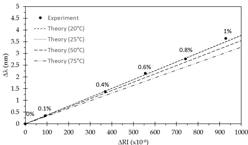
**Figure S1.** Calibration of the SPR measurement set-up using reference solutions (@ 20°C) made of different concentrations of ethylene glycol solutions (% EG by weight in water indicated above each data point).  $\Delta RI$  is the refractive index difference of the solutions to pure deionized water (0%) and  $\Delta\lambda$  is the shift of plasmonic response obtained by centroid calculation.
