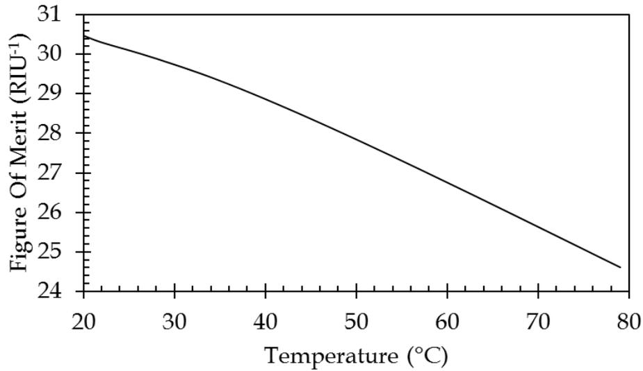
**Figure S4.** Evolution of the Figure of Merit with temperature (modelling)
