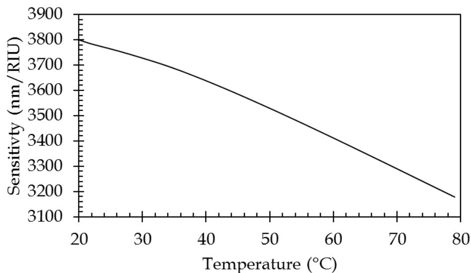
**Figure S3.** Evolution of the sensitivity with temperature (modelling)
