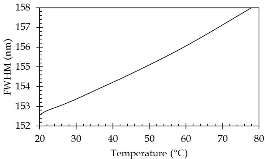
**Figure S2.** Evolution of the FWHM of the plasmonic response with temperature (modelling)
