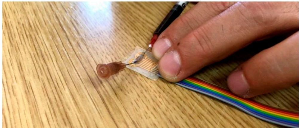
Figure 7. The process of filling the microfluidic channel with electrolyte solution through one reservoir while the air is being released from the second reservoir by a syringe needle.
