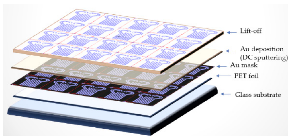
Figure 4. Technological flow for Ti/Au thin film deposition.
