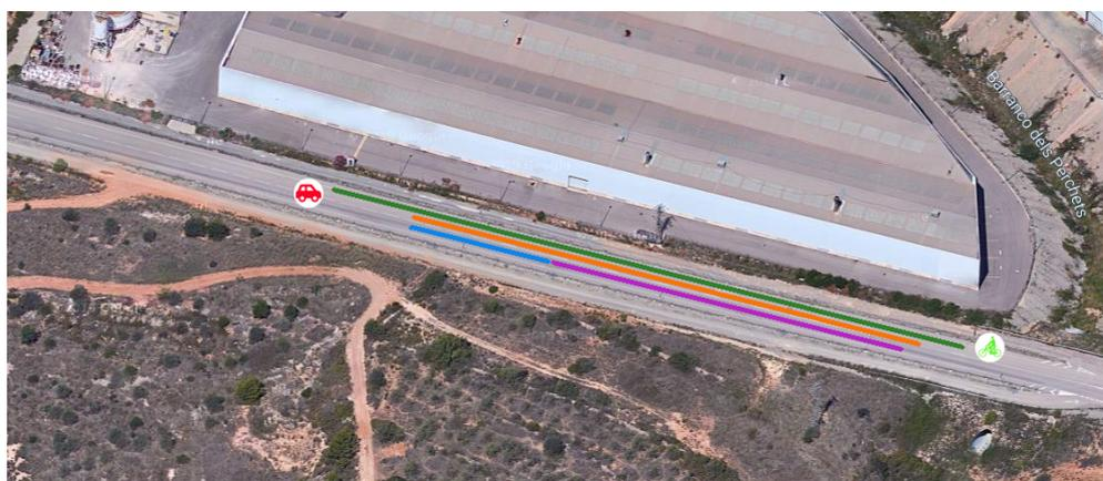
**Figure 18.** Image with distances for the worst case (car and bicycle in opposite directions with a relative speed of 90 km/h). The green line is the alarm threshold (150 m) the orange line shows the distance when the alarm pops up (121 m); the blue line is the car breaking distance (31 m); and finally, the purple line is the remaining distance when the two vehicles are stopped (88 m). Note that the reaction time in the experiment is quite reduced because the driver is waiting for the alarm.
