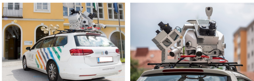
Figure 4. Leica Pegasus Two Ultimate with dual scanner configuration and two pavement cameras (Picture: © Bergmann, 2018).
