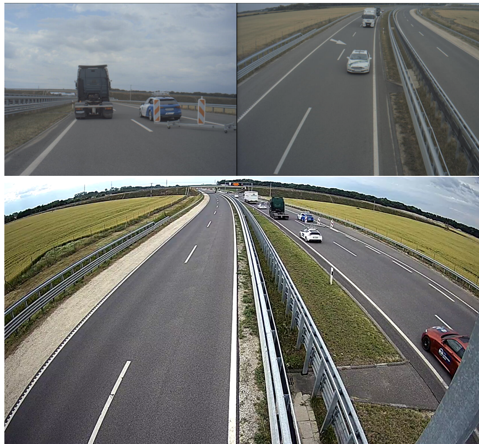
Figure 28. Pictures from the same moment of time from the point of view of the measurement vehicle ( upper left ) and the two infrastructure cameras ( upper right and down ).
