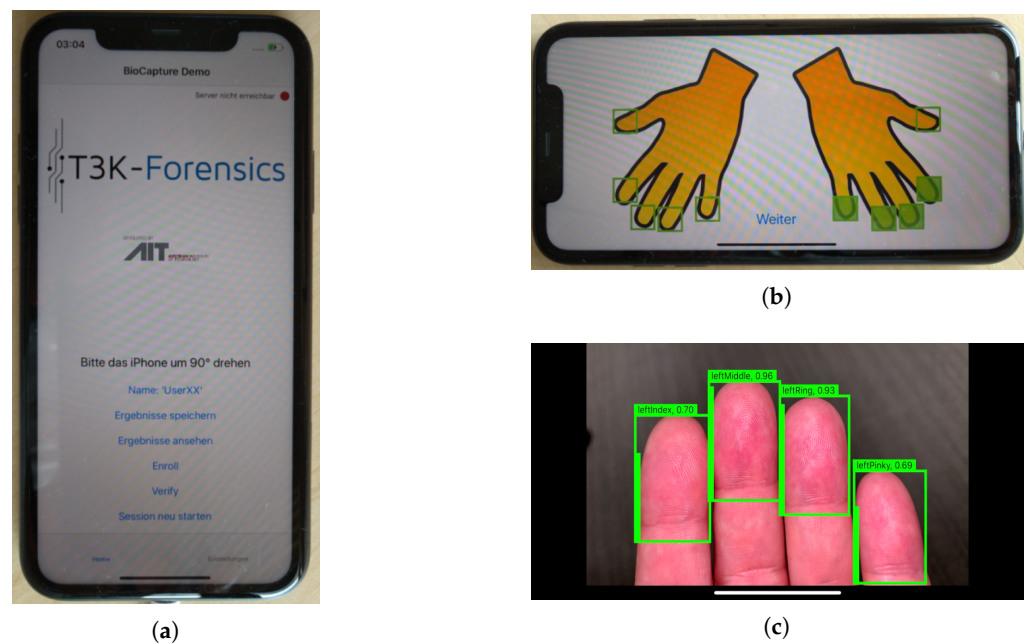
Figure 3. iPhone T3K app example images: (a) user interface, (b) selection of fingers before the acquisition starts, and (c) real-time detection and segmentation of the fingertips. Each fingertip is quantified by a simple quality measure, which is described in Section 2.4. If the FP quality is sufficient, all bounding boxes are colored green before the capturing process ends automatically.
