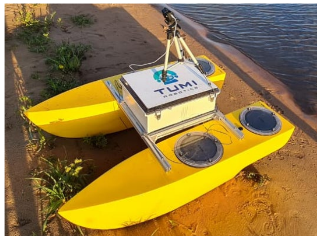
Figure 2. Autonomous Vehicles prototype used in [3] for the monitoring of Ypacaraí Lake. The vehicle has two separate motors and a battery that allows a stable speed of 2 m/s during 4 h of travel.
