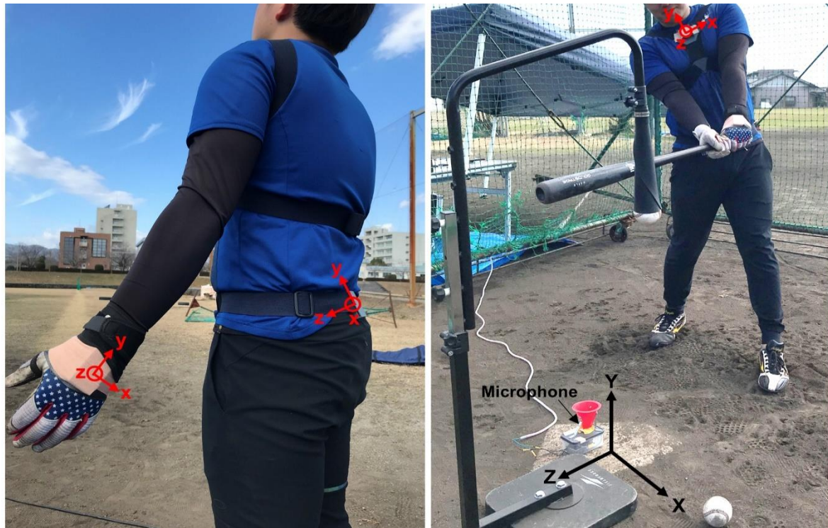
Figure 1. IMU placement and the experimental setup at the tee hitting session. Upper-case letters (X, Y, Z) denote field coordinates, whereas lower-case letters (x, y, z) denote local axes in each IMU attached to the pelvis, thorax, and knob-side hand.
