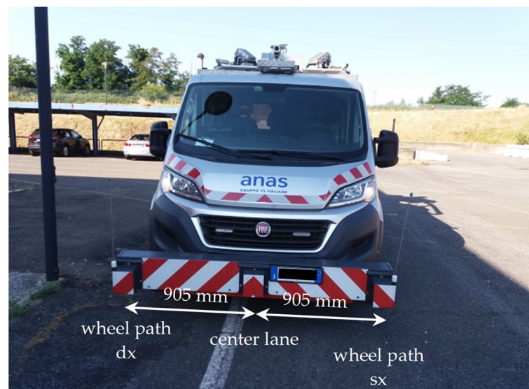
Figure 7. “Cartesio” front view; the RSPs are assembled on a bar in front of the vehicle.
