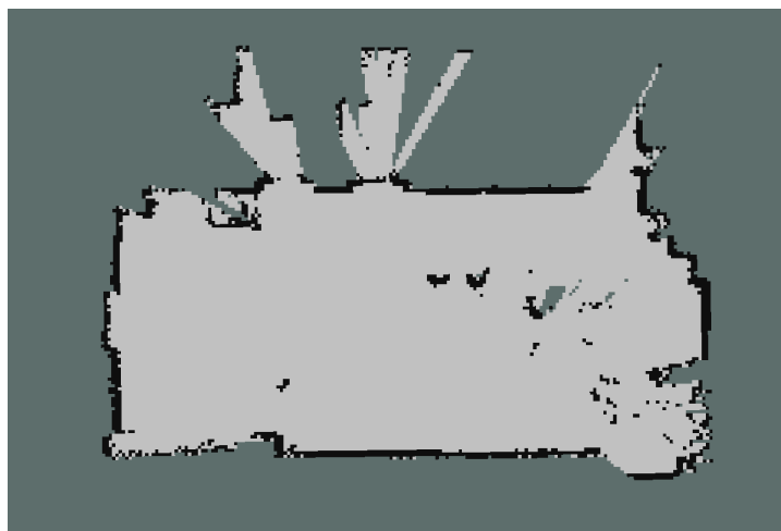
Figure 6. Two-dimensional Occupancy Grid using Gmapping.
