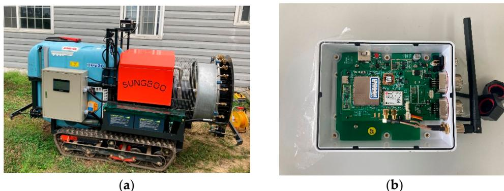
**Figure 2.** Autonomous driving agricultural vehicle (a) and autonomous driving hardware (b).
