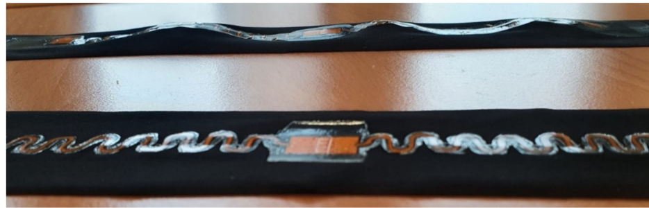
Figure 7. Elasticity difference of V1 and V4 samples. Up: V4 sample after 100 tensile test cycles. The laminated circuit is distorted together with the fabric. Down: V1 sample after 100 tensile test cycles. No distortions into the laminated circuit or fabric were seen.
