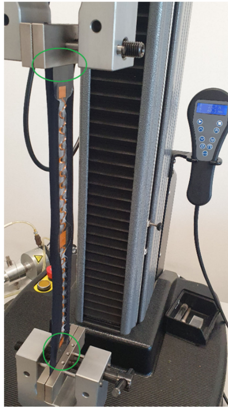
Figure 2. Stretched sample where the green circled areas highlight that the sample was clamped from the laminated fabric area and not just fabric.
