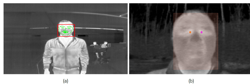
Figure 7. Examples of samples where semiautomatic label technique was applied. (a) Automatic Labeling. Red rectangle refers to bounding box of identified face, and green dots to respective facial marks. (b) Manual labeling. Orange rectangle is associated to identified face, while orange and violet dots refer, respectively, to points that identify right- and left-caruncles.
