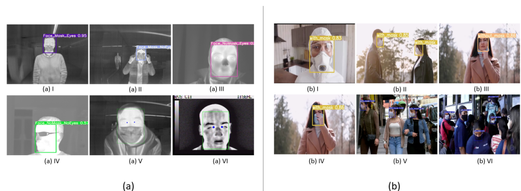
Figure 11. (a-I - a-VI) Examples of results obtained in images, from inference of selected algorithms for mask and glasses detection components and detection of zone corresponding to human caruncle. (b-I - b-VI) Examples of results obtained in images, from inference of selected YOLOv5 algorithm for mask detection.
