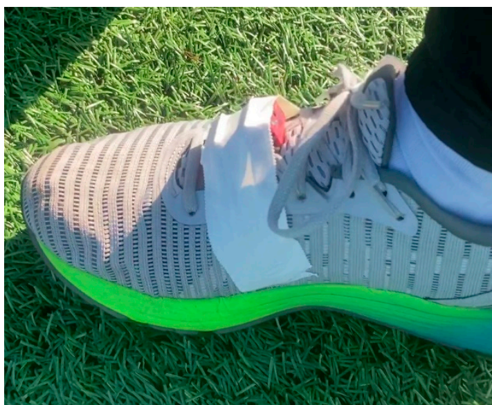
Figure 1. Attachment of the IMU on the instep.
