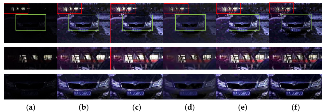
Figure 11. (a) Test image and its detail maps. The remaining images are the enhancement results and their detail maps, generated by the following methods: (b) ALSM, (c) Li et al. [26], (d) LR3M, (e) LIME, and (f) the proposed method.
