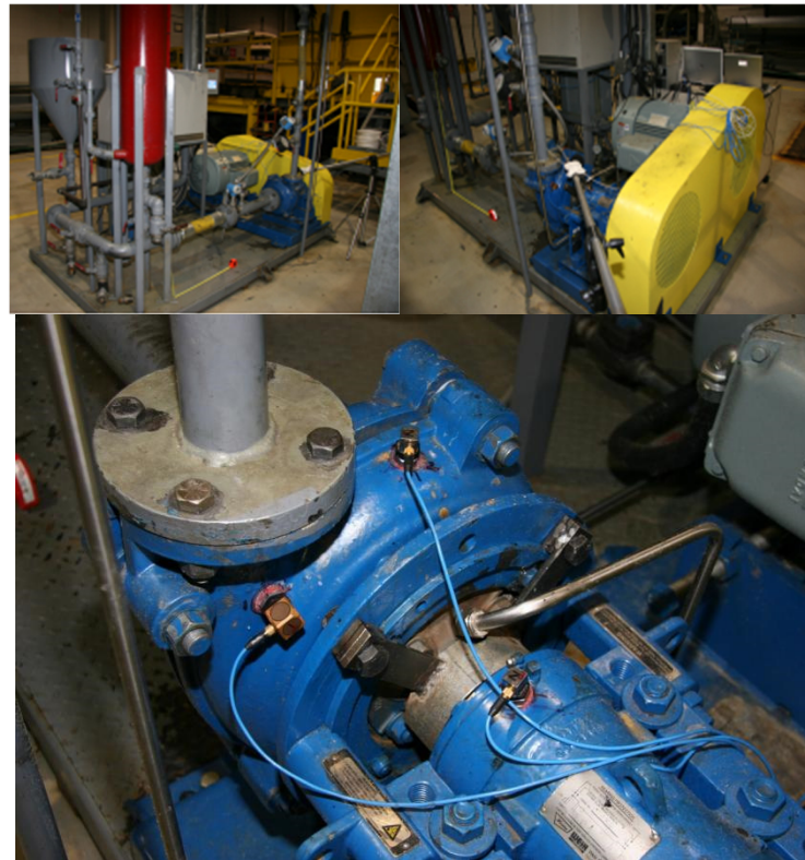
Figure 3. Experimental system of slurry pump with multiple channel sensors.
