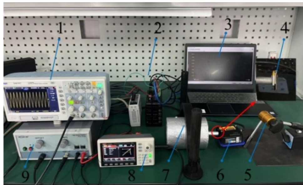
Figure 22. The experimental platform (1. Oscilloscope, 2. Controller, 3. PC, 4. Attitude Sensor 5. Magnetic Base, 6. Laser Sensor, 7. Prototype, 8. Signal Generator, 9. Voltage Amplifier).
