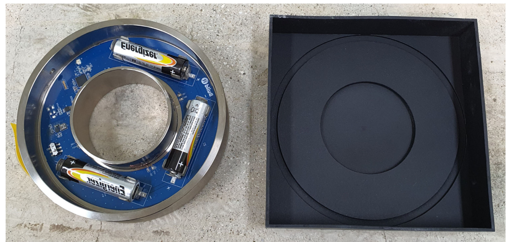
Figure 12. Wireless Bluetooth load-cell prototype and rubber casing.
