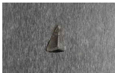
Figure 2. Pyramid attached to the falling film surface as an example of a film disturbance.
