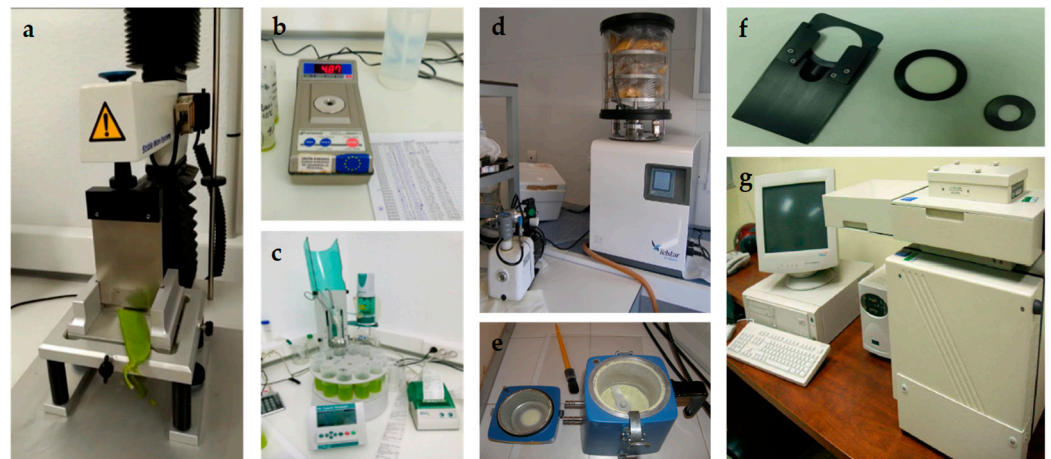
Figure 3. Detail of Texturometer XTPlus Texture Analyzer (a); Smart-1 digital refractometer (b); Automatic Metrohm 862 Titrosampler (c); Freeze-drying equipment (d); Mill (e); NIRS sample holder (f); Spectrometer Model 6500 Foss-NIRSystems (g).
