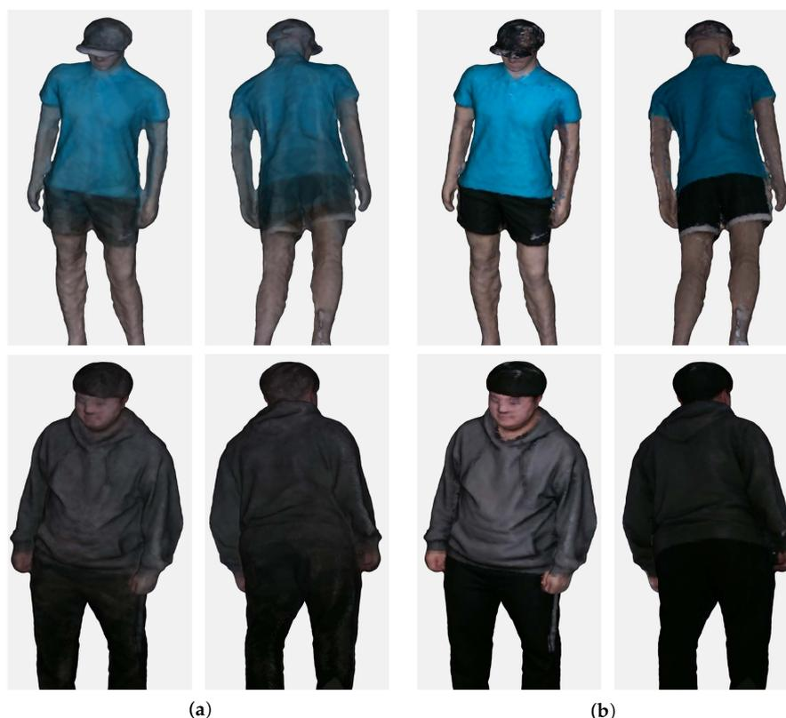
**Figure 8.** Colored 3D meshes. The 3D meshes are reconstructed using depth maps estimated by the Census stereo matching method. The median color mapping shows more reliable and accurate results than average colors. (a) Mean; (b) Median.
