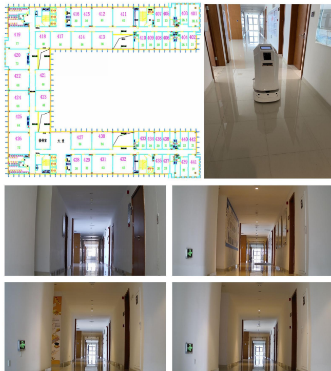
Figure 6. The layout of the experimental corridor environment, the mobile robot constructing DB_W and DB_I , automatically, and several image samples from DB_I .
