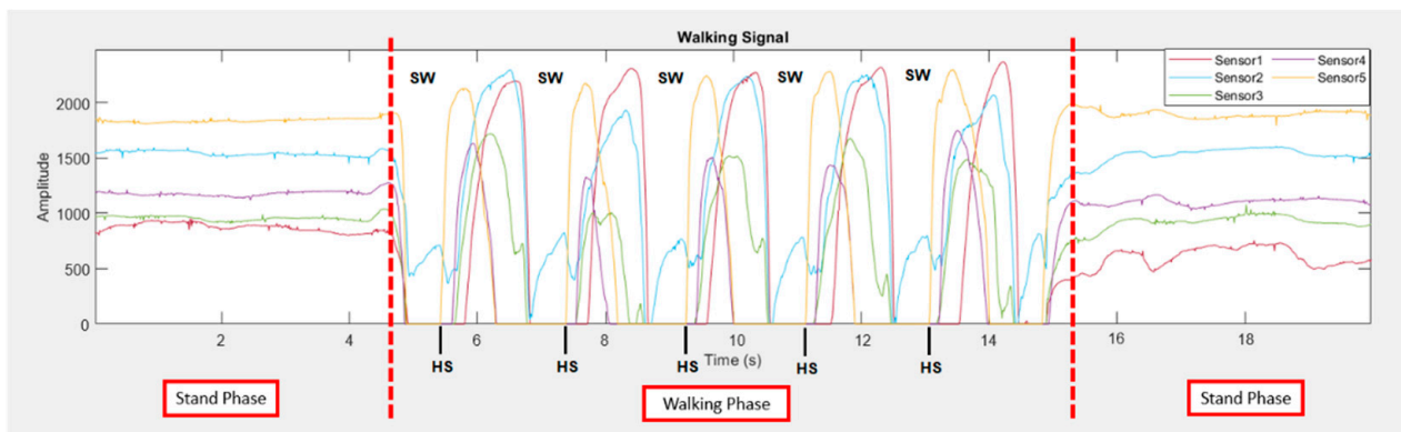
Figure 3. Examples of measured signals from five sensors. (SW: swing, HS: heel strike).
