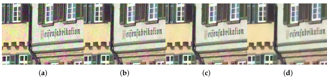
Figure 9. Influence of regularization parameter \lambda_1 for test image House for crosstalk degradation 2 (crosstalk kernel with \sigma_g = 0.6 and noise with \sigma_n = 0.04 ): (a) \lambda_1 = 0.01 , (b) \lambda_1 = 0.03 , (c) \lambda_1 = 0.05 , and (d) \lambda_1 = 0.1 .
