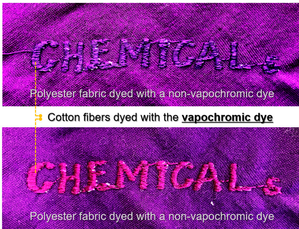
Figure 6. Visualization of the concept of textile-based vapor sensor.
