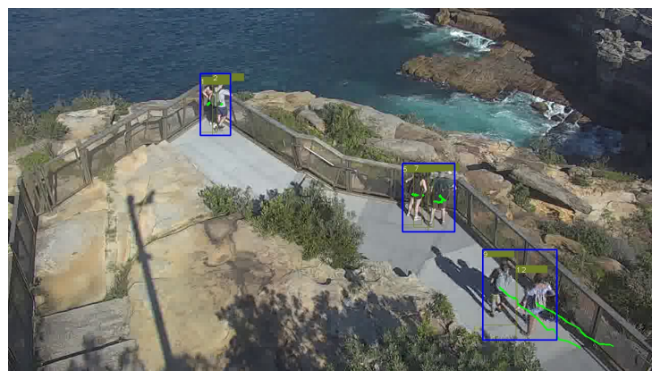
Figure 2. Demonstration of the trajectory analysis API: grouping and trajectories for a duration of 2 s (60 consecutive frames) with trajectories been shown in green.
