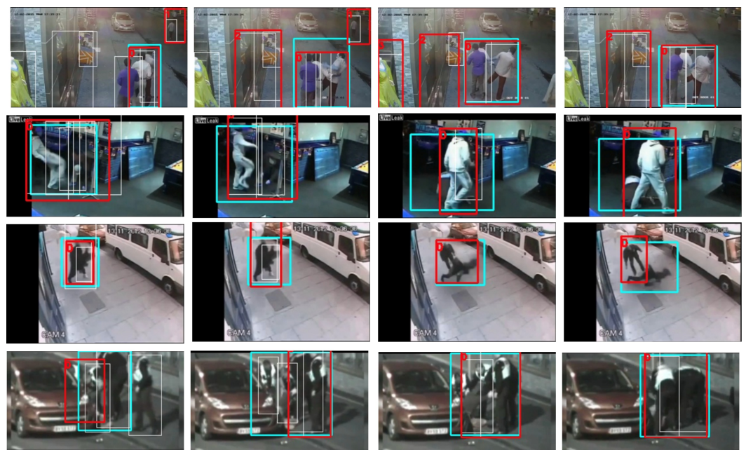
Figure 9. Video samples from the UCFCrime2Local dataset with person detections (white boxes), ground truth (light blue boxes), and action tubes (red boxes).
