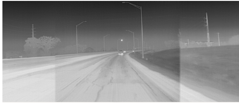
Figure 2. Thermal cameras are resilient to direct sunlight. Showing the same scene as in Figure 1. Reprinted with permission from earlier conference paper Ref. [11]. ©2021, SAE International.
