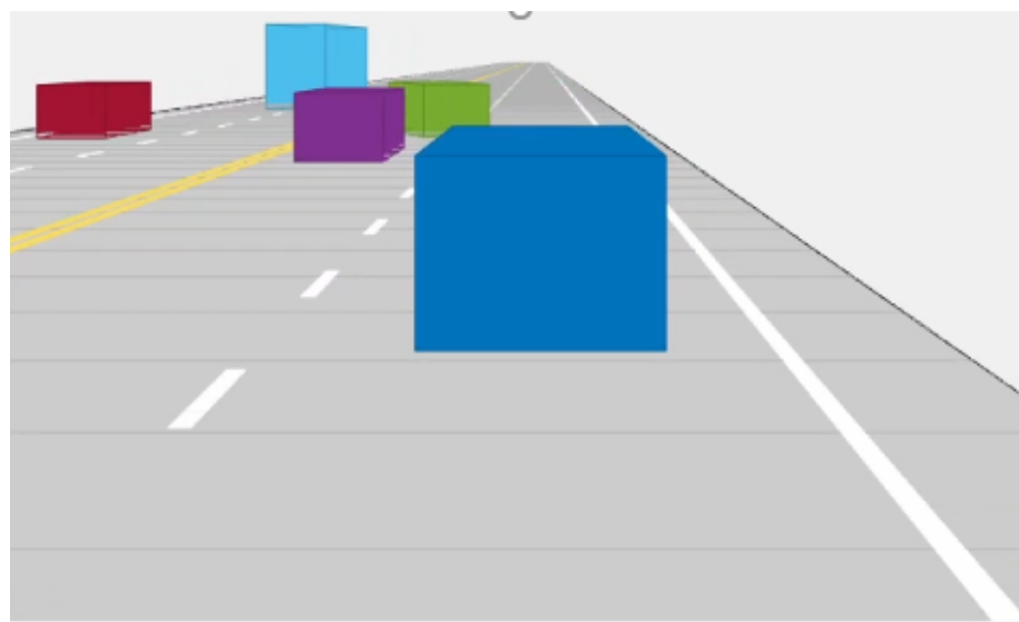
Figure 13. A screenshot of the scenario designed in Driving Scenario Designer. Each color shows a different vehicle.
