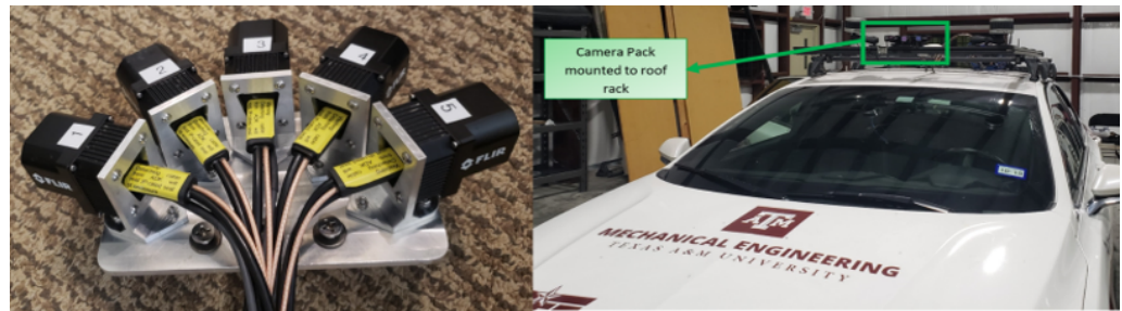
Figure 4. Thermal camera assembly. Each of the five thermal cameras used for the image stitching are shown with the numbers 1–5.
