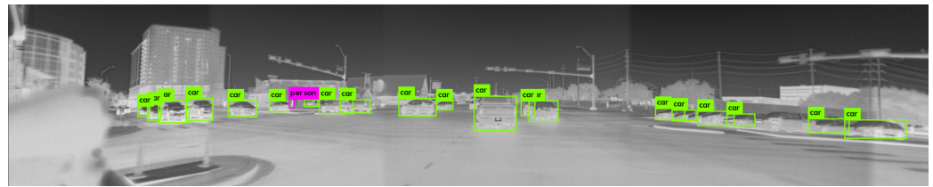
Figure 8. An example of the output of the object detector running on the thermal images.
