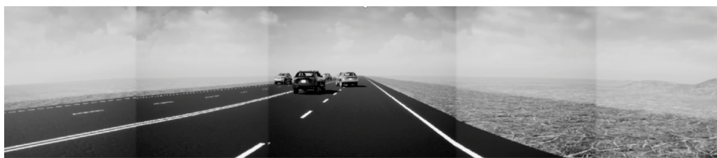
Figure 14. A screenshot showing a virtually generated panorama, as seen through simulated cameras, from the ego vehicle. Image is in gray-scale to reflect the output type of thermal images.
