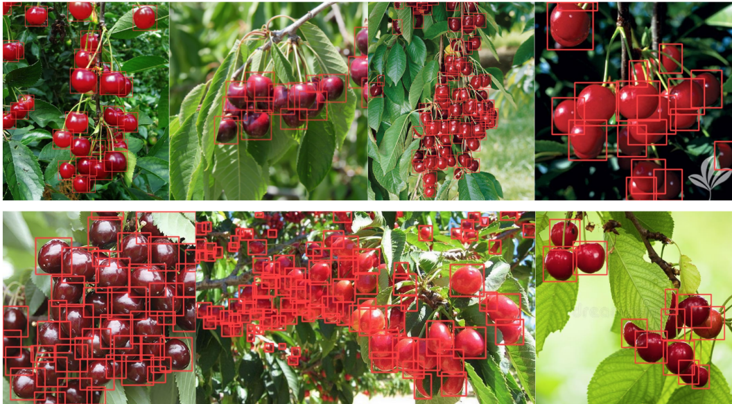
Figure S5. Cherry prediction results using Yolov5x and RGB test images that achieved 0.66 mAP_{[0.5:0.95]} . Images are obtained from Google Images.
