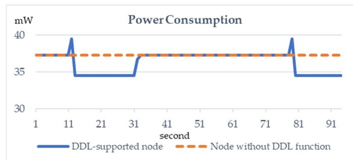
**Figure 10.** The change in standby power consumption of two nodes.
