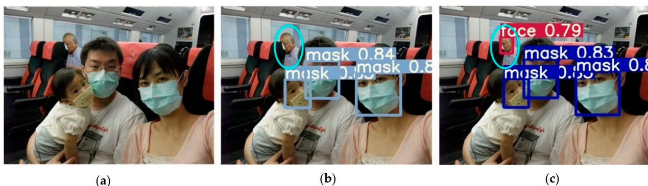
Figure 14. Detection of obscured targets. (a) Initial image sample; (b) YOLOv5 detect results; (c) YOLOv5-CBD detect results.
