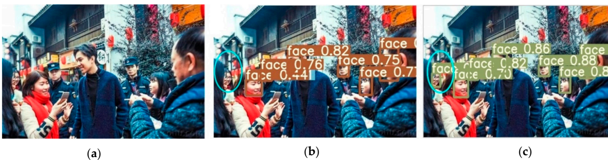
Figure 15. Detection of cross-dense targets. (a) Initial image sample; (b) YOLOv5 detect results; (c) YOLOv5-CBD detect results.
